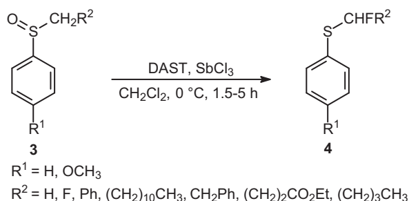
Scheme 3. Synthesis of \alpha -fluoro sulfides 4 from sulfoxides 3 with DAST under \text{SbCl}_3 catalysis.
